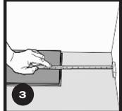
At the end of the first row, leave an expansion gap of 1/4" (6mm) to the wall and measure the length of the last plank to fit.
