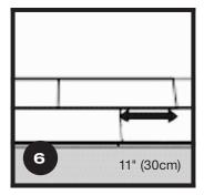
Make sure that end joints of all planks should be staggered 30cm at least or more.
