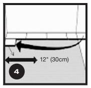
Start the second row with the leftover cut part of the last plank of the previous row. This small plank should measure at least 12" (30cm). Otherwise, cut a new plank in half and use it to begin the second row. Whenever practical, use the piece cut from the preceding row to start the next row.
