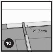
The last row of floorboards should be at least 2" (5cm) wide. If needed reduce the width of first row.
