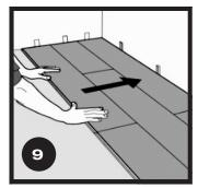
After the first 2-3 rows of planks are installed, they should be checked with a string line to ensure that rows are still running straight. If they are not, it could be that the starting wall has some irregularities that caused bowing in the installation.
