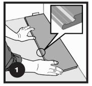
After thoroughly cleaning the subfloor, you should begin laying from left to right. Position the first plank so that grooved edge is facing you. Use a spacer to set a 1/4" (6mm) gap between flooring and the wall.
