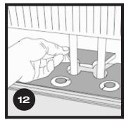
When drilling holes around a vertical object, make sure the holes are bigger than the width of object, cutting the small area and filling into the inner side.
