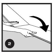
Second plank, first row. Drop the plank of short side first, and then gently tap down the end with a rubber mallet so it firmly locks into the previous plank until both are at the same height. Make sure both planks are perfectly aligned. Continue installing the first row until you reach the wall on the right.
